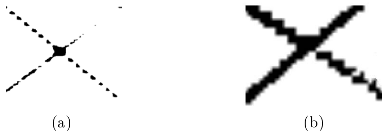
Figure 2.3: Improper thresholding of lines: (a) underthresholding causes corrupted and non-continuous lines. (b) overthresholding leads to lines spanning multiple pixels
