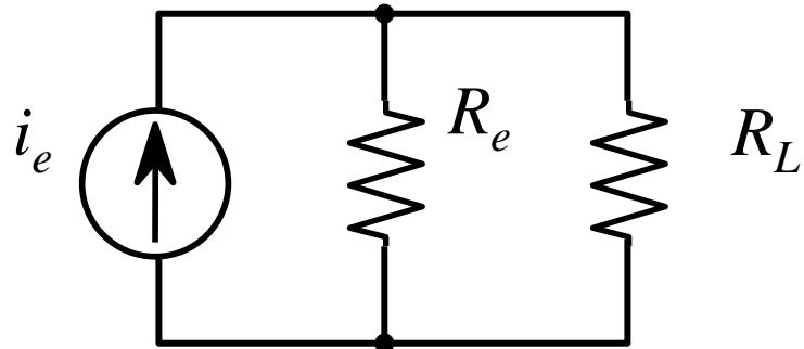
$$i_e = V_L \left( \frac{1}{R_e} + \frac{1}{R_L} \right)$$
