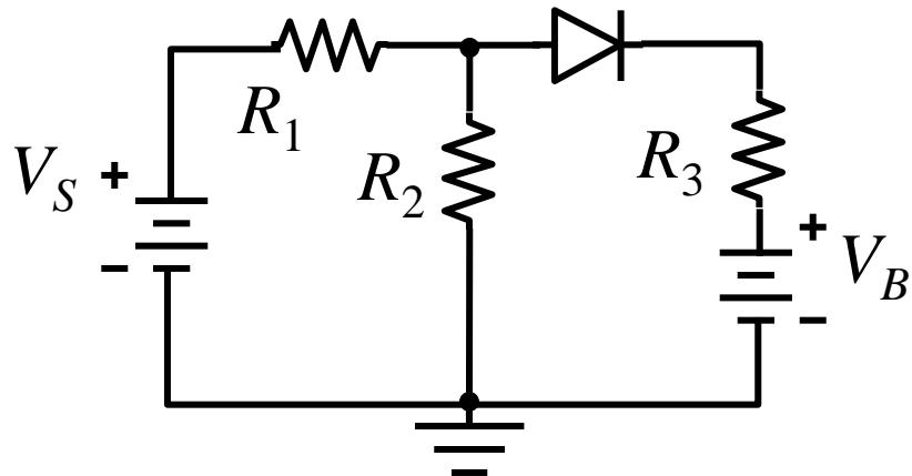
$$\begin{aligned}V_S &= 12 \text{ V} \\R_1 &= 2 \Omega \\R_2 &= 10 \Omega \\R_3 &= 6 \Omega \\V_B &= 9 \text{ V}\end{aligned}$$
