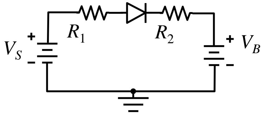
$$\begin{aligned}V_S &= 12 \text{ V} \\R_1 &= 5 \Omega \\R_2 &= 8 \Omega \\V_B &= 10 \text{ V}\end{aligned}$$
