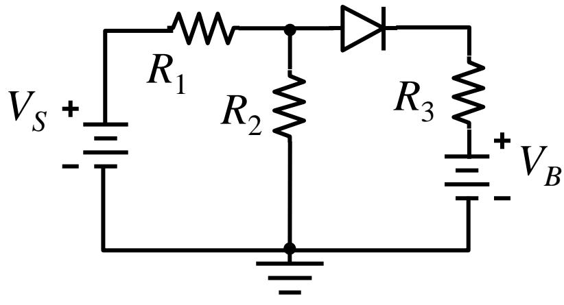
$$\begin{aligned}V_S &= 12 \text{ V} \\R_1 &= 2 \Omega \\R_2 &= 10 \Omega \\R_3 &= 6 \Omega \\V_B &= 9 \text{ V}\end{aligned}$$
