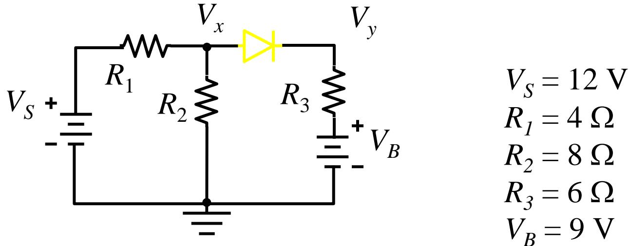
$$V_x = \frac{R_2}{R_1 + R_2} V_S \quad V_x = \frac{8}{12} \cdot 12 = 8$$
