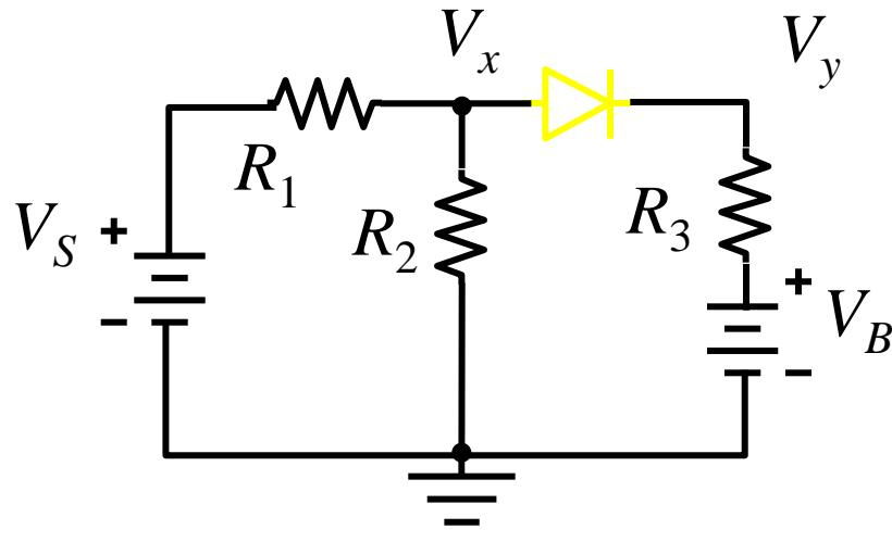
$$\begin{aligned}V_S &= 12 \text{ V} \\R_1 &= 2 \Omega \\R_2 &= 10 \Omega \\R_3 &= 6 \Omega \\V_B &= 9 \text{ V}\end{aligned}$$
