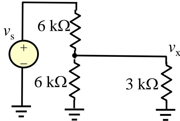
$6 \text{ k}\Omega \parallel 3 \text{ k}\Omega = 2 \text{ k}\Omega$ .
