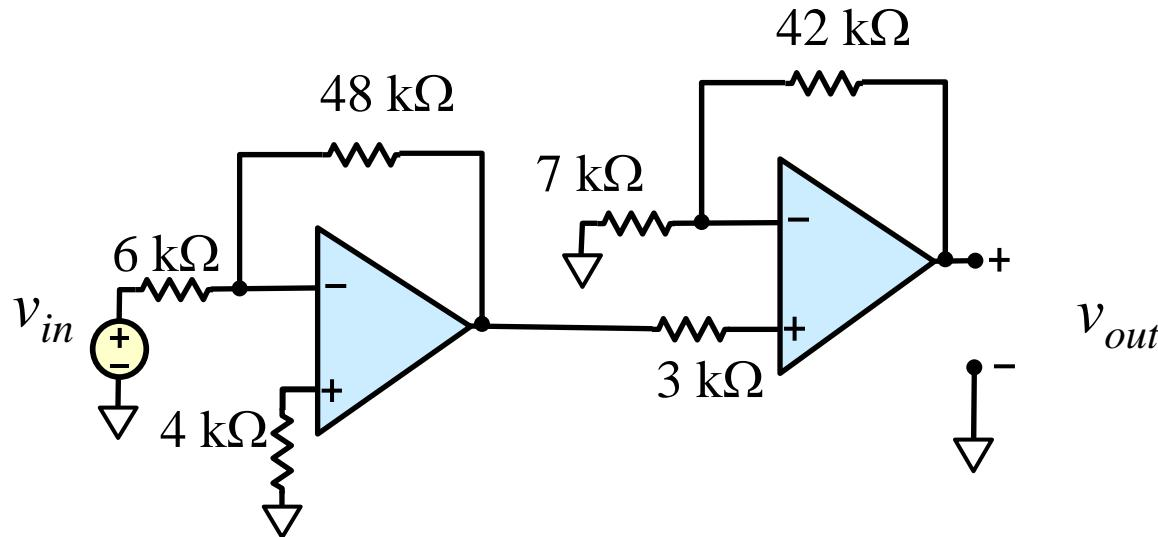
Find the gain  $\frac{v_{out}}{v_{in}}$
