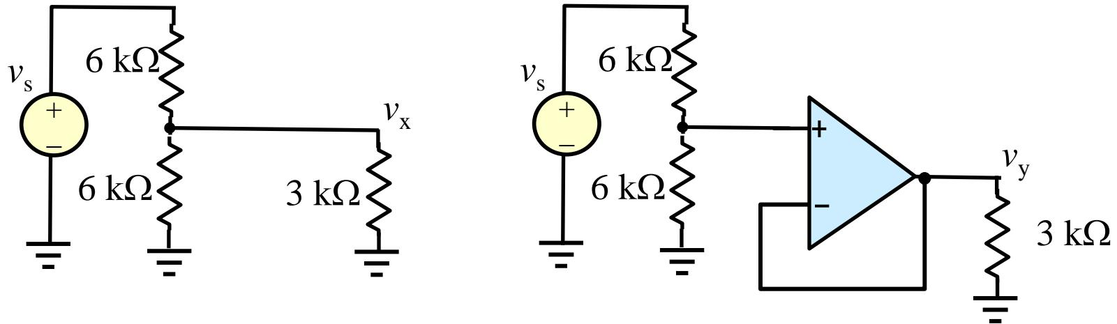
Find  $v_x$  (left diagram) and  $v_y$  (right diagram) if  $v_s = 12 \text{ V}$ .
