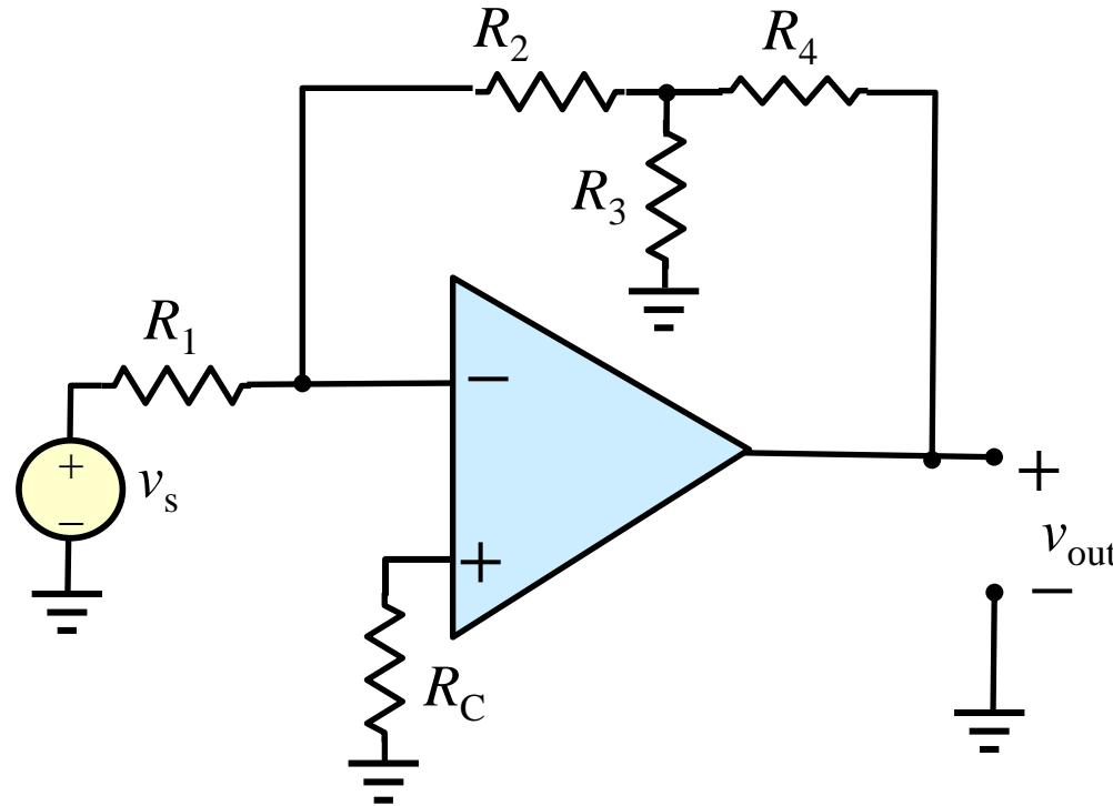
Find the voltage gain if  $R_1 = R_3 = 1 \text{ k}\Omega$  and  $R_2 = R_4 = 10 \text{ k}\Omega$ .
